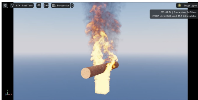
Figure 11: Scene with a Fire Smart object bound to a cube preset and an Unknown Smart Object bound to a cylinder marked as nonflammable.
